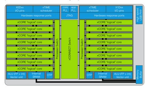
Figure 1: XU316-1024-QF60B block diagram
