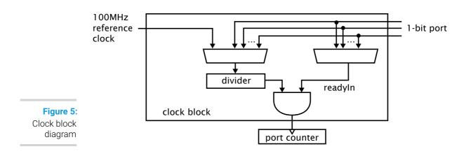
On reset, each port is connected to clock block 0, which runs from the xCORE Tile reference clock.
