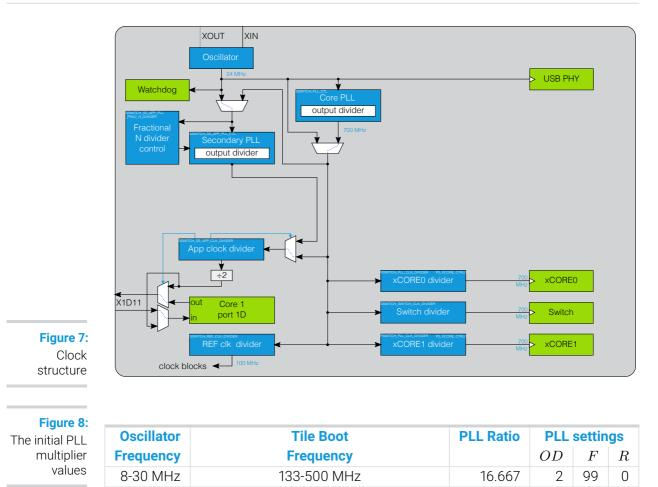
Figure 8 lists the oscillator frequency range, and the values of OD, F and R, which are the registers that define the ratio of the tile frequency to the oscillator frequency:
