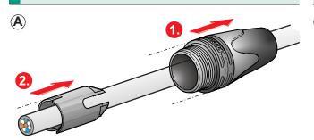
(A) Slide the boot (1.) and the chuck (2.) onto the cable.
