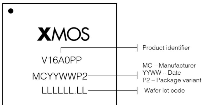
Figure 1-1 Part marking scheme
