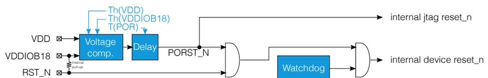
When the device comes out of reset, the boot procedure starts (Section 9). The chip can be reset externally using the RST\_N pin. If required, the JTAG state machine can be reset to its idle state by clocking TCK five times whilst TMS is high.
