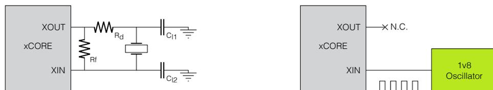
$R_f$  should be  $1M\Omega$ . Calculation of  $C_{l1}$ ,  $C_{l2}$  and  $R_d$  are beyond the scope of this datasheet, and we recommend that you use a crystal with characteristics as specified in Table 11. These have an ESR of at most 60 Ohm, have a load capacitance of 12 pF, and all resonate at their fundamental frequency.
