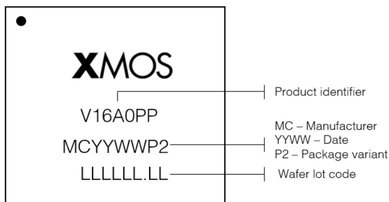
Figure 1-1 Part marking scheme
